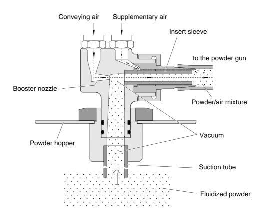
The concentration of the powder/air mixture, and with it, the powder output depends on the conveying air pressure and supplementary air pressure, the quality of the powder, the length of the powder hose, the diameter of the powder hose, the number of coils in the hose, the difference in the height between the gun and injector, and the type of nozzle. The condition of the insert sleeve is of great importance, because wear causes the powder output to sink drastically.
